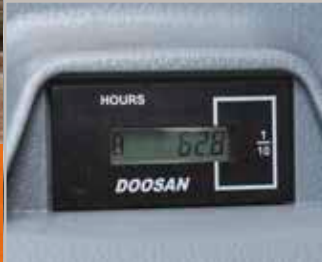
Hour meter (from ground level)
