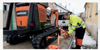
**Transportability:** The DX10Z fits easily on a conventional trailer. Easier transportability with new integrated upper structure tiedown points.
