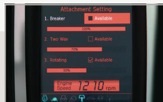
Attachment: selectable auxiliary hydraulic flow settings
