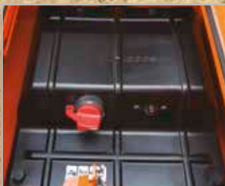
Battery cut-off switch
