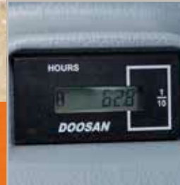
Hour meter (from ground level)
